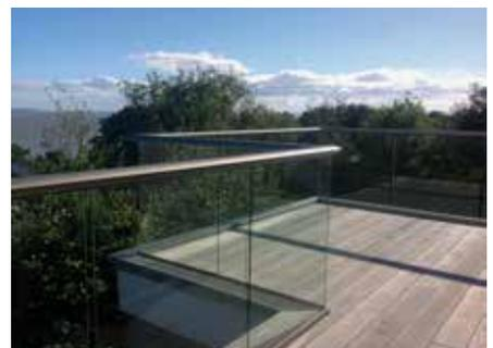
either side to a wall or structural element. The Aerofoil handrail provides the longest post-free spans of up to 4m without posts. Both systems include panels of 10mm toughened glass, which can be produced in a variety of tint options including the standard clear, and customised blue, grey, bronze, green, and satinised (opaque).
